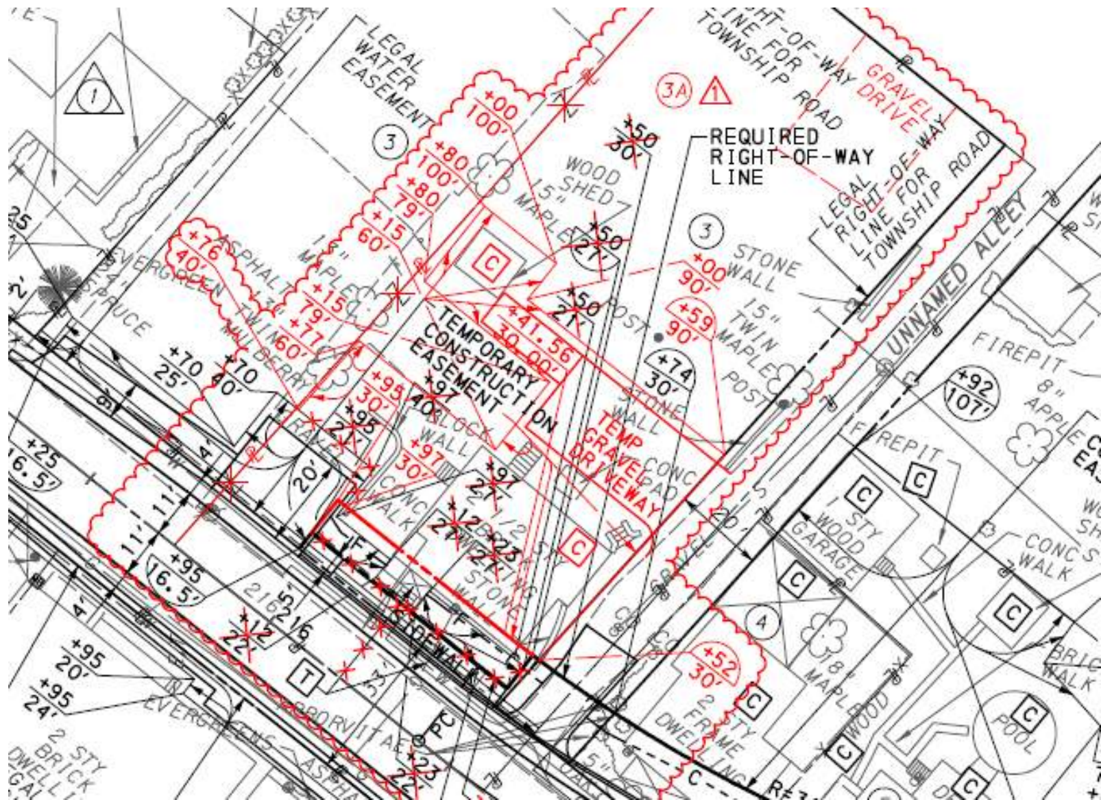
Revised ROW plan required to remove house and relocate driveway.
